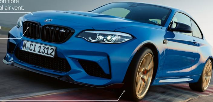
Front splitter in carbon fibre.
