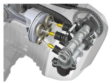
Via an axial displacement of the intake camshaft, the intake valves are actuated by either the partial-load cam or the full-load cam, depending on the load and speed. The axial displacement of the intake camshaft and thus the use of partial-load or full-load cam is established via a shift gate on the camshaft and an electromechanical actuator that is engaged there.
