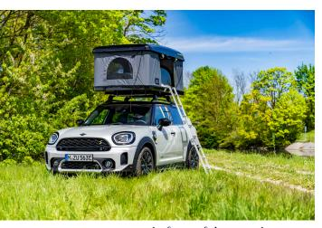
The shelter can be erected at dizzy heights within a few seconds. After releasing the safety catches on the housing, the tent structure lifts up automatically with the help of gas springs. The eight rungs of the foldout aluminium ladder can be climbed just as quickly. Inside, there are two comfortable sleeping berths. In summer heat, the windows can be rolled up, and thanks to the mosquito
