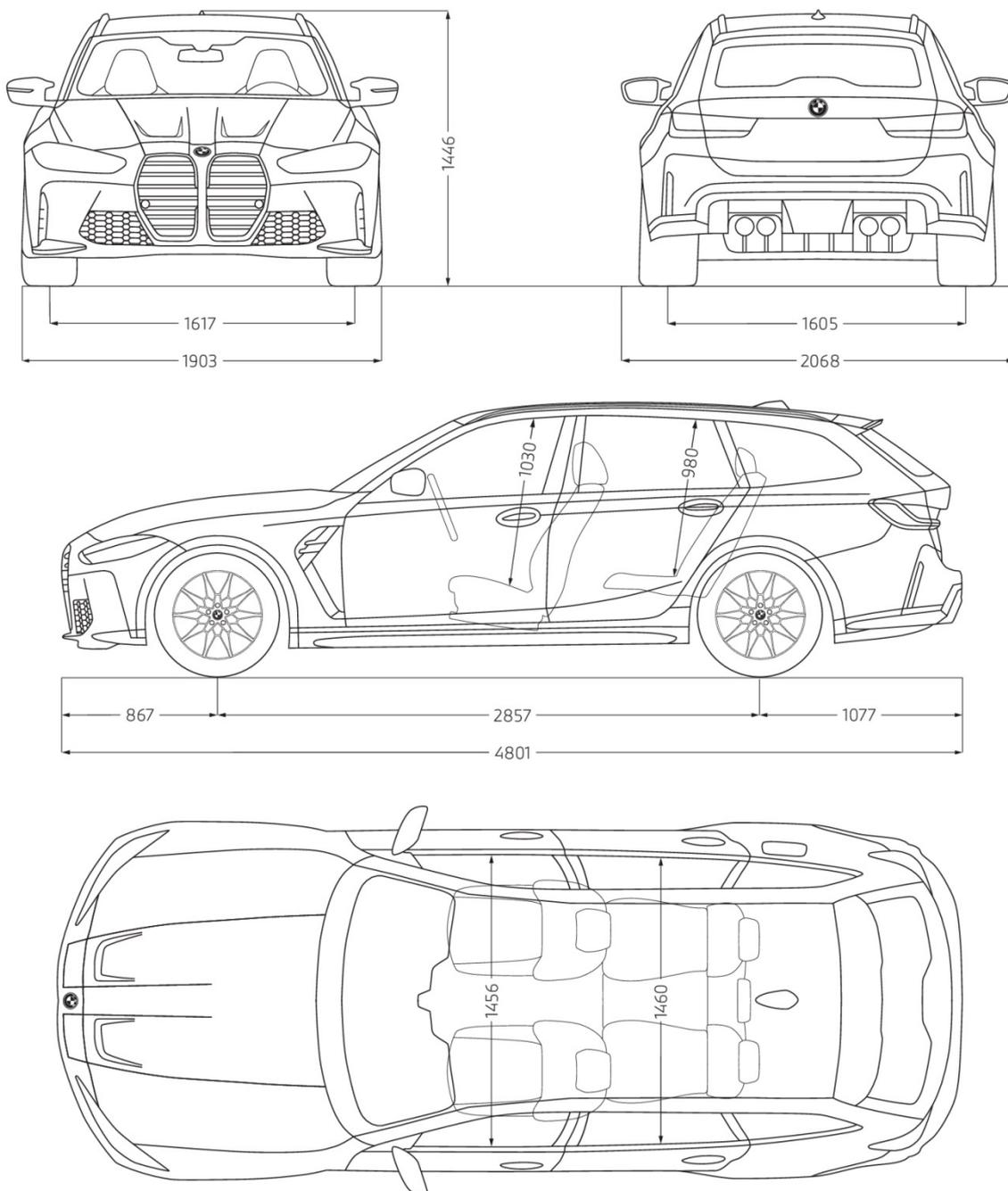
The dimensions of the technical drawings are in millimetres and may vary depending on the model and optional equipment.
