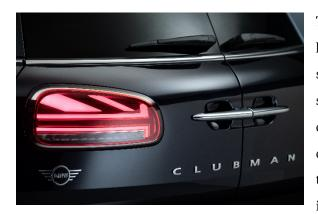
The new MINI Clubman is also fitted with LED rear lights as standard. The light units with chrome surround are especially integrated in the wings of the split door. The rear lights feature a horizontally oriented design that underscores the brand's British origins: the graphic structure of their light sources traces the abstracted pattern of the Union Jack. With its striking lines, the flag motif provides a distinctive
