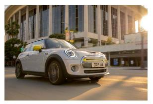
Part of the characteristic driving experience in an electrically powered BMW Group model is the one-pedal feeling. The vehicle perceptibly decelerates as soon as the driver removes their foot from the accelerator. This effect occurs when the electric motor performs the function of a generator in coasting mode; kinetic energy transforms into electric power, which is in turn fed back into the
