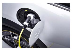
The charging connection of the new MINI Electric is designed for alternating current (AC) and direct current (DC) charging using Type 2 and CCS Combo 2 plugs. Above the connection, a charge level indicator displays orange signals for initialisation, a pulsating yellow light for an ongoing charging operation, and a green light for a fully charged battery.
