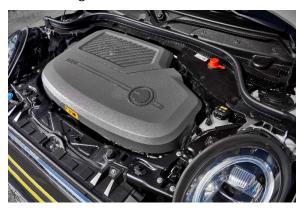
Spontaneously initiated drive torque and continuous power delivery without gear shift interruption – these are the characteristic features of the drive technology fitted in the new MINI Electric. They ensure hallmark MINI driving fun in a novel form that offers a particularly intense experience. The power source is the latest, highly powerful version of the synchronous electric motor developed by the BMW Group.
