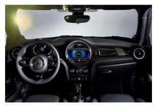
The new MINI Electric is fitted as standard with a 5.5-inch digital instrument cluster in. At the centre of this fully digital screen, the road speed is shown in figures with a peripheral scale band. The speed band is also displayed in the light ring of the central instrument according to the mode selected – in red (SPORT mode), white (MID) or green (GREEN and GREEN+).
