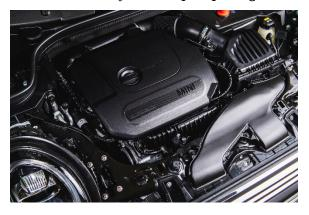
The 3-cylinder petrol engine of the MINI One Piccadilly Edition draws its power from a capacity of 1.5 litres, with a maximum power output of 102 hp and a top torque output of 190 Nm. The potent engine features petrol direct injection with a maximum pressure of 350 bar, ensuring that drivers can zip through the ins, outs, and roundabouts of Singapore with effortless flair. The engine has been developed
