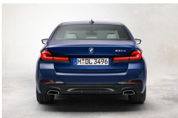
Black edging and a new L-shaped graphic give the rear lights of the new BMW 5 Series additional visual impact. The rear lights and brake lights are integrated into a shared light fixture, which now forms a single unit with the prominently three-dimensional external lens. Regardless of the
