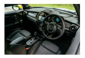
In addition, a 5-inch digital screen behind the steering wheel is fitted as standard. This digital instrument cluster was first seen on the MINI John Cooper Works GP, and is now available on all variants across the range. It displays all driving-relevant information as well as check-control messages and status displays of the driver assistance systems.
