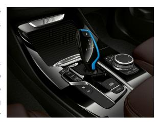
This adaptive recuperation is automatically engaged when the gear lever is in 'D' mode. For a higher level of battery recuperation, the driver just needs to shift the gear lever to 'B' mode – this would allow for the one-pedal operation that is familiar from the i3.
