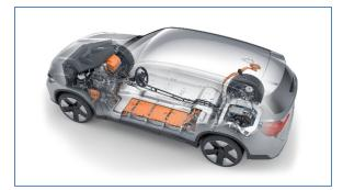
In the iX3, we have a 400V lithium-ion battery – this consists of 188 prismatic battery cells in 10 modules. This modular concept means that each cell is individually housed and controlled for longevity and the highest possible level of safety.
