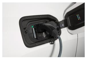
The Combined Charging Unit (CCU) in the first-ever BMW iX has been designed to offer a very high level of charging flexibility. DC power can be taken on board at a rate of up to 150 kW. This allows the battery's state of charge to be increased from 10 to 80 per cent in around 31 minutes. What is more, range can be increased by more than 95 kilometres in just ten minutes when it is plugged into a DC fast-
