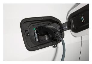
The Combined Charging Unit (CCU) in the first-ever BMW iX has been designed to offer a very high level of charging flexibility. DC power can be taken on board at a rate of up to 150 kW. This allows the battery's state of charge to be increased from 10 to 80 per cent in around 31 minutes. What is more, range can be increased by more than 95 kilometres in just ten minutes when it is plugged into a DC fast-
