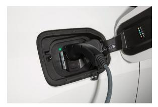
The Combined Charging Unit (CCU) of the first-ever BMW i4 has been designed to enable extremely flexible battery charging. DC charging is possible at up to 205 kW. For example, in a short mid-journey stop at a high-power charging station, the car's range can be increased by as much as 164 kilometres within 10 minutes from a 10 per cent charge level.
