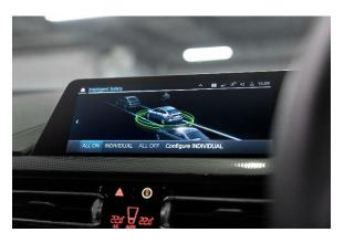
The Driving Assistant package is also fitted as standard – this comprises of the Lane Change Warning system, which prompts the driver to guide the car back onto the correct lane by means of a visual warning and, if necessary, a steering input. Other functions include the route-ahead assistant, rear collision warning and crossing traffic warning, which reduces the risk of a collision when
