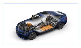
In the same vein as the BMW i4 eDrive40, the BMW i4 M50 shares the same fifth-generation BMW eDrive technology and offers a highly integrated electric drive system. The electric motors are free from rare-earth materials as it does not require the use of fixed permanent
