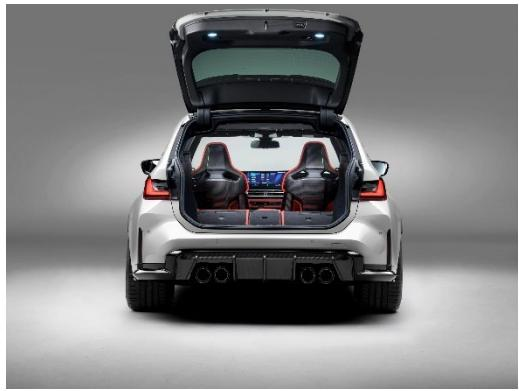
The rear compartment of the first-ever BMW M3 Touring has three full-size seats. The rear-seat backrest can be split 40 : 20 : 40. Folding down individual seat sections or all of them at the same time allows the car's load capacity to be expanded from 500 litres to a maximum 1,510 litres, as required. Automatic tailgate operation and the
