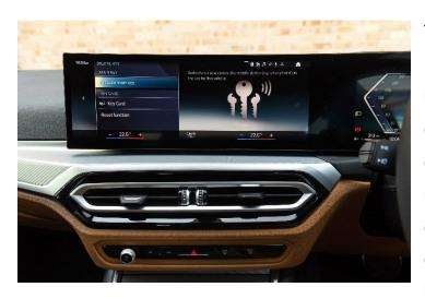
The Comfort Access feature on the BMW 3 Series Touring provides keyless access to the vehicle. For additional convenience, the driver is able to set the car to automatically unlock when approaching the vehicle, and correspondingly, lock when the driver is moving away with the vehicle key. The driver is also able to
