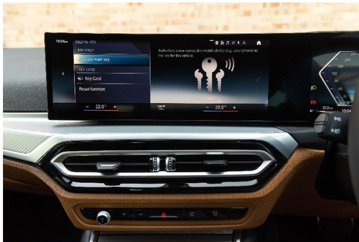
The Comfort Access feature on the BMW 3 Series Touring provides keyless access to the vehicle. For additional convenience, the driver is able to set the car to automatically unlock when approaching the vehicle, and correspondingly, lock when the driver is moving away with the vehicle key. The driver is also able to
