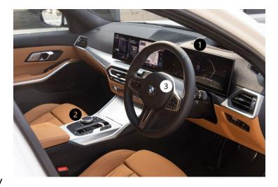
comprises of a 12.3-inch digital instrument cluster and a 14.9-inch central infotainment system. Drivers are also able to see pertinent information in their line of sight with the full-colour Head-up Display available as standard.
