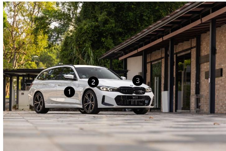
2. The standard adaptive LED headlights with blue accent strips feature slim contours and daytime driving lights arranged in an inverted L-shape. The outer daytime driving light elements also serve as turn indicators. The adaptive headlights' range of functions includes the cornering light and non-dazzling matrix high beam, as well as dynamic headlight range control and variable light distribution.
