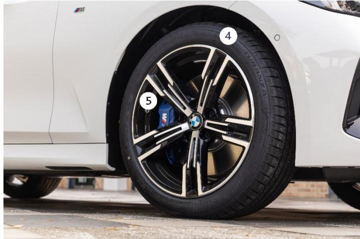
5. As part of the M Sport Pro package, the BMW 3 Series Touring is fitted with M Sport brakes including blue-painted callipers with the 'M' inscription. The brakes provide increased thermal stability and a sporty brake pedal feel.
