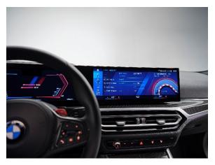
The new BMW M2 boasts a driver-centric cockpit featuring M-specific readouts and controls plus setup options. On the advanced BMW Curved Display, driving-related information including Shift Lights appears in a new graphical layout on the 12.3-inch information display. M-specific widgets for vehicle setup and tyre condition are just two of the items that can be called up in the
