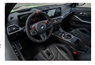
speed M Steptronic transmission with Drivelogic. This is operated using either the M-specific selector lever on the centre console, or the carbon-fibre shift paddles on the Alcantara-wrapped steering wheel. The driver can use the Drivelogic button integrated into the selector lever to alter the transmission's shift characteristics, with the choice of comfort-oriented, sporty and track-optimised settings.
