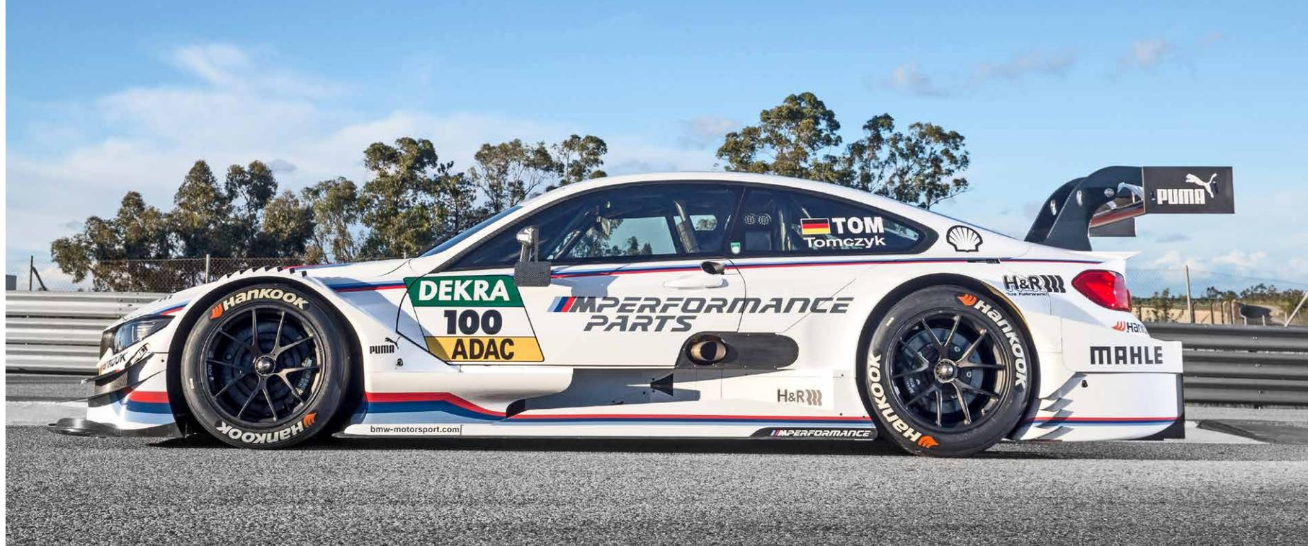
use of two air restrictors with 28 millimetre diameters, meant little time was required to determine the speeds to be expected. The designers were then able to derive basic data like the configuration of the suction funnels and the exhaust system.
