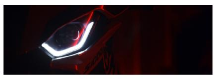
The front turn indicators are no longer mounted in the trim but integrated in the rear mirror instead. The new and in particular higher positioning of the turn indicators means the RR is now even more visible to other road users. By the same token, it takes no time at all to get the RR ready for track use. The "Comfort Indicator" function is a new feature. Here, the turn indicator automatically goes into neutral position so the rider can't forget it.
