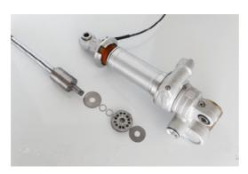
The DDC damping valves in the predecessor model were connected in series. The volume flow passed through the conventional and electrically adjustable damping section. Conventional damping was the lowest level of damping available. The electrical DDC valve increased damping. However, this resulted in the familiar drawback that the compromise between comfort and high damping tended to cause underdamping and pumping of the suspension.
