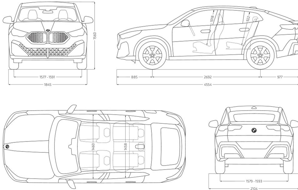
The dimensions indicated in the technical drawing are in millimetres and may vary depending on the model and the items of optional equipment fitted.
