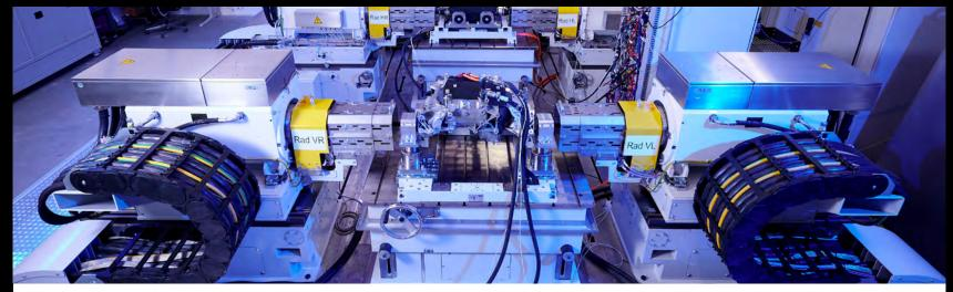
development work at BMW never stands still – and it is getting faster all the time. The E-Drive system test rig plays a central role here, helped by what is arguably its most impressive feature: the ability to test parts that are not yet available in finished product form by simulating them as virtual components. Together with increased process efficiency, this serves to shorten the development time for innovations by as much as one-and-a-half years.
