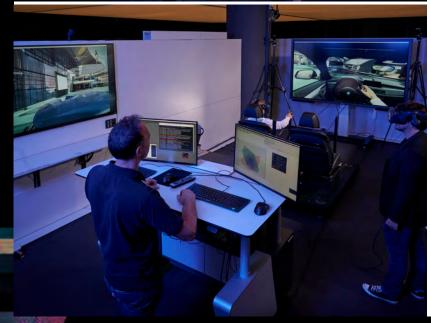
in this area, BMW employed a reusable interior design. The use of rapid prototyping – a fast-paced process for manufacturing sample components – adds a mixed-reality dimension to the development process. I.e. it benefits from the intelligent combination of surfaces you can actual feel and control elements presented using virtual reality.
