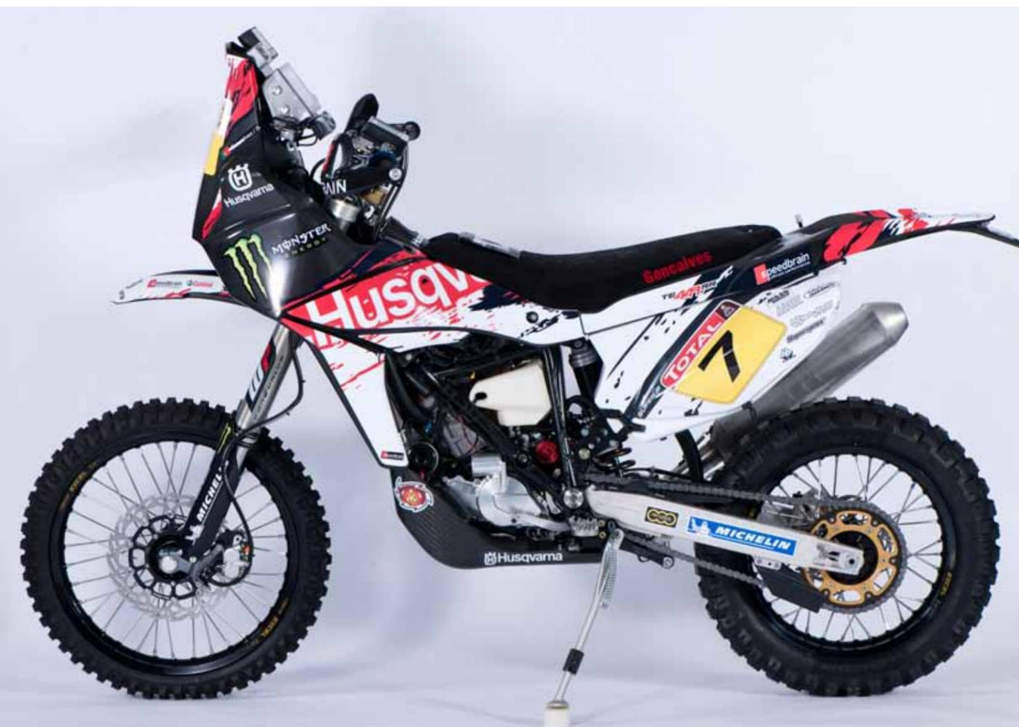
Water-cooled, 4-stroke single-cylinder engine, two overhead camshafts, four valves, dry sump lubrication with oil cooler, electronic intake pipe injection / digital engine management
