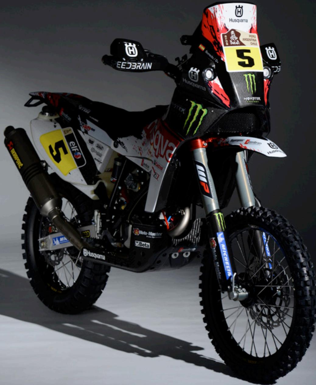
Water-cooled, 4-stroke single-cylinder engine, two overhead camshafts, four valves, dry sump lubrication with oil cooler, electronic intake pipe injection/digital engine management
