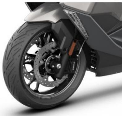
At the front, a twin disc brake with a diameter of 270 mm and two radially bolted 4-piston floating calipers with a piston diameter of 28 mm ensure powerful and stable deceleration. Rear wheel deceleration is taken care of by a single disc brake with a diameter of 270 mm and a single-piston floating caliper with a piston diameter of 32 mm. High-quality braided steel brake lines are used to achieve a stable pressure point and optimum controllability.
