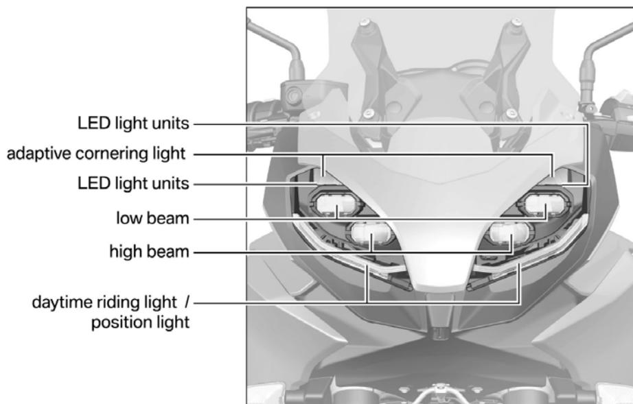
**Adaptive Cornering Light – unique in the mid-range – part of Headlight Pro as an ex works option. Powerful LED lighting units all round as standard.**
