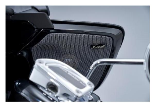
The new R 18 B and R 18 Transcontinental are equipped with a standard sound system developed together with the British manufacturer Marshall featuring two 2-way loudspeakers, each with 25 watts output, integrated into the front fairing, black speaker grills and white Marshall lettering. In the standard audio system offers an exhilarating sound experience.
