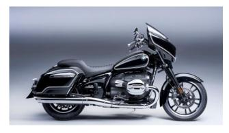
With a low fairing windshield and a short, narrow two-person seat as well as a long dynamically elegant down-sloping line, the new R 18 B embodies the typical "bagger" style. The engine is finished in metallic matte black as are the black fork and fork sleeves, as well as black rear-view mirrors, handlebar
