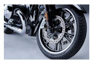
The R 18 B and R 18 Transcontinental feature cast light alloy wheels. The  $3.5 \times 19$ -inch front wheel is equipped with a  $120/70 \times 19$  or  $120/70 \times 19$  tire (depending on the manufacturer), while a  $180/65 \times 16$ -inch rear wheel. Original BMW Motorrad Accessories offers additional rims in chrome, Machined or 2-Tone-Black.
