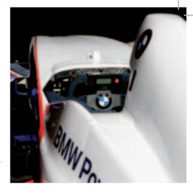
the optimum shift point. while an LCD display gives information on such things as water temperature, oil pressure, engine speed, selected gear and the last or best lap time. Standard equipment also includes a data recording device that allows the driver and the engineer to achieve the optimal set-up and further improve the driver's style.
