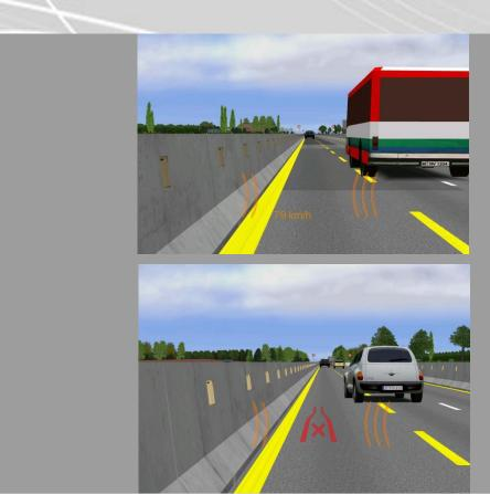
Measures the effectively available width of the road Displays the lateral clearance on left and right side Feedback for the driver on which side there is less clearance to the barrier or vehicle. (0,5 - 1,0 meters)
