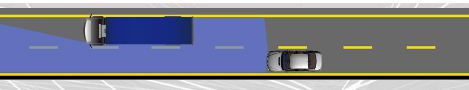
Activation together with lane departure warning Lane departure warning orients towards yellow road markings Measures the effectively available width of roadway (preSite) Measures the clearance to barriers and to other vehicles (inSite)
