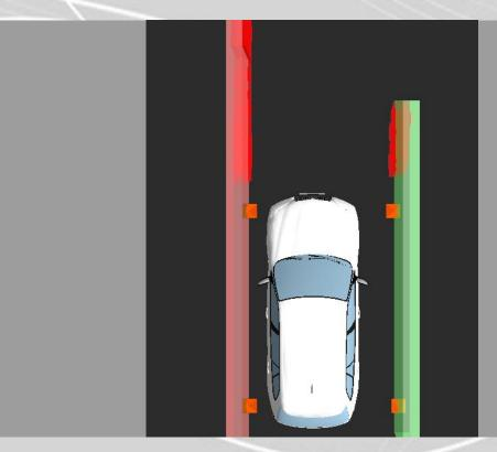
Monitors the lateral clearance while passing the constriction
