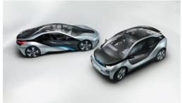
The impressive swathes of exposed CFRP reflect the lightness and efficiency of both vehicles. As a central element of efficient mobility, aerodynamics play a key role in reducing fuel consumption. The design of the BMW i vehicles uses numerous aerodynamic measures to reduce the cars' drag substantially, increasing their efficiency – and therefore their range when running on electric power alone.
