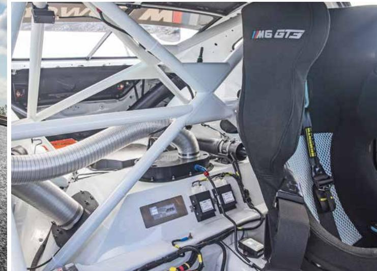
the BMW wind tunnel. Priority was given to ensuring maximum driver safety. To offer the drivers of the BMW M6 GT3 as much protection as possible against the effects of an accident, BMW Motorsport itself developed and produced the FIA-approved safety cell in accordance with the very latest safety standards. The engineers also placed great importance on efficiency and ease of maintenance, as well as reliability, which is particularly crucial at the 24-hour classics.
