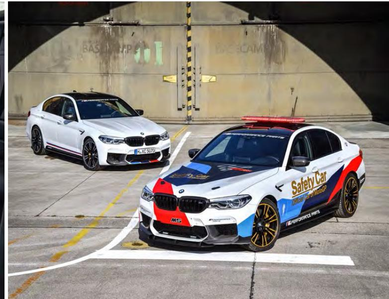
The transformation of the BMW M5 to a MotoGP Safety Car was completed by the inclusion of special racing features and the necessary safety equipment. The front splitter is a prototype developed specifically for the BMW M5 MotoGP Safety Car and the bonnet latches are taken directly from racing. The bucket seats from the BMW M4 GTS guarantee a combination of comfort and maximum security for their occupants while in action on the racetrack.
