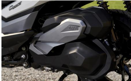
The entire drive unit of the new BMW mid-size scooter has been completely newly developed and includes a directly integrated CVT gearbox as well as a secondary drive in the form of a drivetrain swing arm. The liquid-cooled single-cylinder engine has a capacity of 350 cc, derived from an 80 mm bore and a 69.6 mm stroke. Its rated power output is 25 kW (34 hp) at 7 500 rpm and the maximum torque of 35 Nm is reached at 6 000 rpm. The maximum engine speed is 8 800 rpm.
