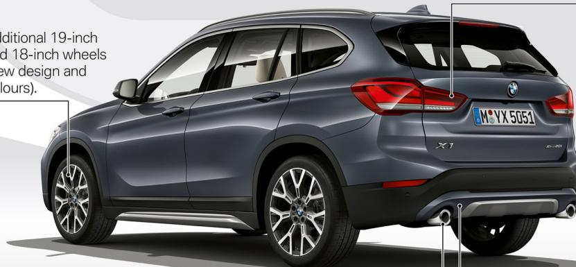
Diameter of exhaust tailpipes increased from 70 to 90 mm.
