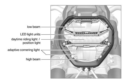
"In the F 900 R and F 900 XR, the Adaptive Cornering Light enters the mid-range. Iconic light guides with daytime riding light function give both models a strong sense of character and recognisability. Combined with all-round LED lighting and the standard TFT screen with connectivity, the R and XR clearly stand out from the crowd." Stefan Kollar, Electrical Development
