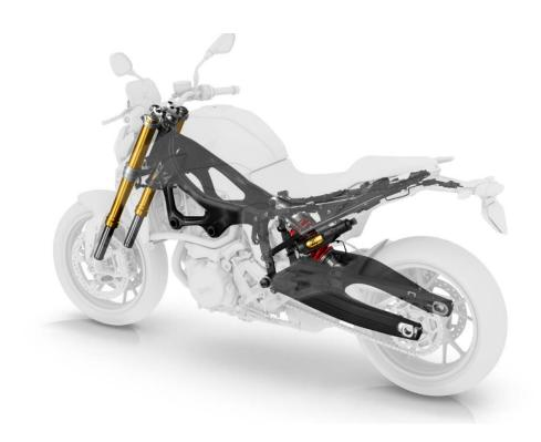
"By adjusting the steering head angle, offset and castor, we were able to achieve a particularly sporty suspension design for the road models. Optimum design of the respective ergonomic triangles allows pronounced segment-specific differentiation while at the same time offering great possibilities in terms of individualisation". Wolfgang Wallner, Suspension Development
