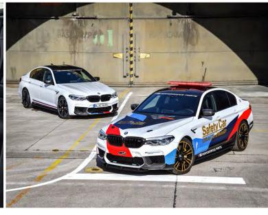
The transformation of the BMW M5 to a MotoGP Safety Car was completed by the inclusion of special racing features and the necessary safety equipment. The front splitter is a prototype developed specifically for the BMW M5 MotoGP Safety Car and the bonnet latches are taken directly from racing. The bucket seats from the BMW M4 GTS guarantee a combination of comfort and maximum security for their occupants while in action on the racetrack.
