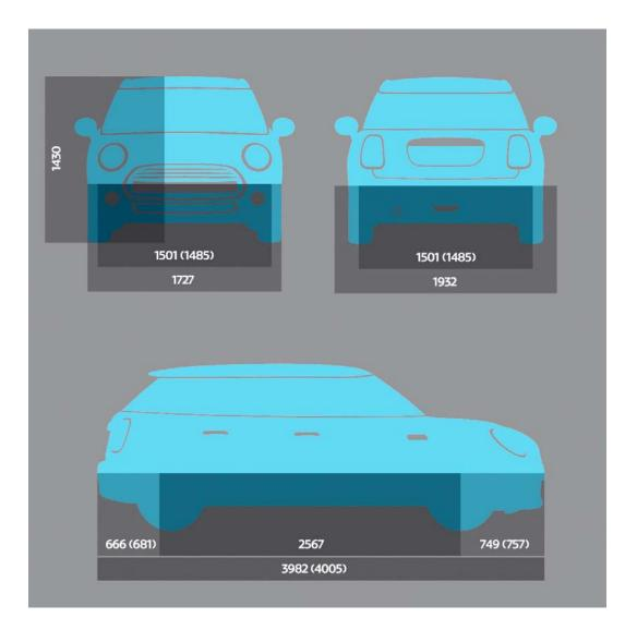
Dimensions in mm apply to MINI Cooper 5 door (figures in brackets apply to MINI Cooper S 5 door and MINI Cooper SD 5 door)
