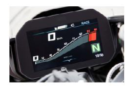
In addition to an expanded range of functions and information, the BMW Motorrad developers attached particular importance to excellent readability of the 6.5-inch TFT screen. For optimum visibility even in difficult light conditions, the screen was therefore designed to be large for good readability. It is linked to the Multi Controller on the left-hand handlebar panel and can be operated quickly, safely and conveniently from here.
