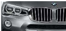
552 - FULL LED ADAPTIVE 5AC - HIGH BEAM ASSIST
