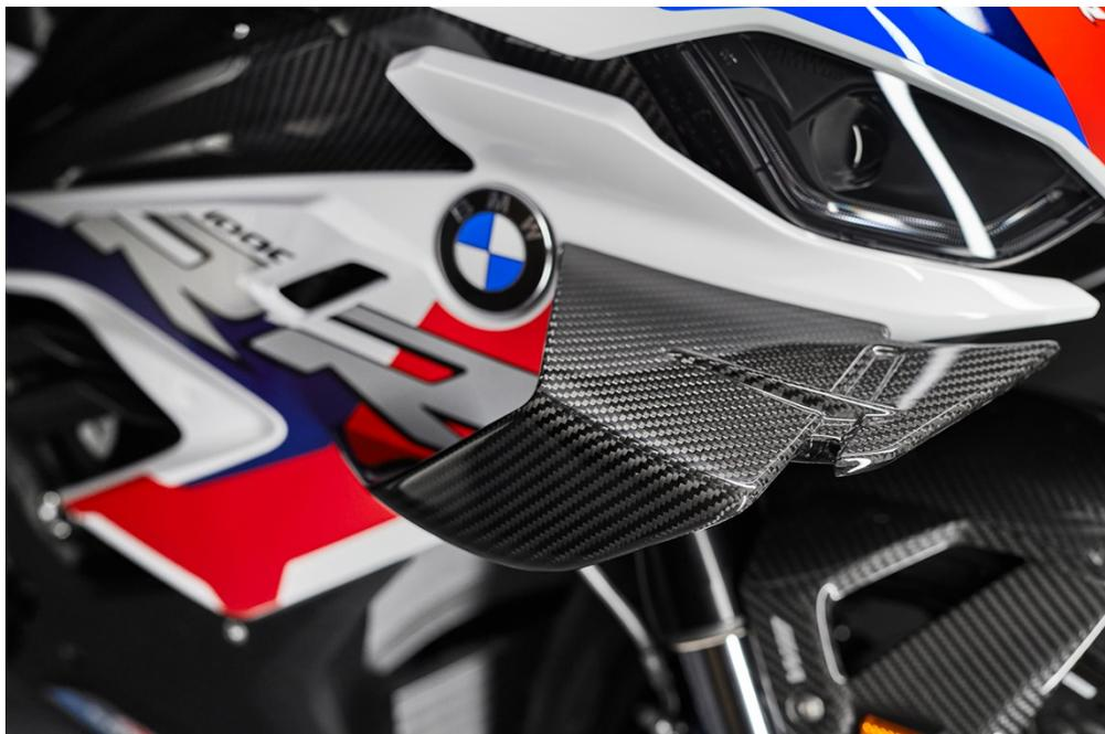
The development work for the M winglets took place during test drives on the race track and also in the wind tunnel of the BMW Group. The following downforce values were determined for the front and rear sections of the new M RR:
