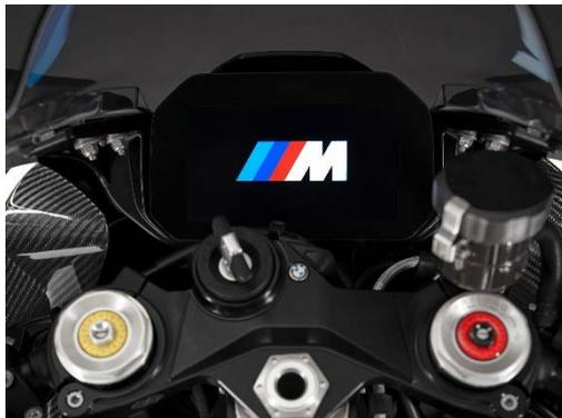
The instrument cluster of the new M RR has the same basic design as the RR and has an M start animation. As part of the optional equipment, an activation code (contents of M competition package) can be used to provide comprehensive data material for the use of the M GPS laptrigger and M GPS data logger (Original BMW Motorrad Accessories) via the OBD interface of the instrument cluster.
