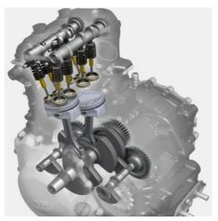
While the oscillating mass forces of the previous models were compensated for by a connecting rod fitted to the middle of the crankshaft with a defined arrangement of counterweights, unwanted vibrations in the new engine are eradicated by means of two counterbalance shafts.
