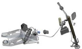
Unlike conventional suspension systems – i.e. those that are not electronically controlled, Dynamic ESA Pro taps into a whole new dimension of ride safety, performance and comfort since the damping is automatically adapted
