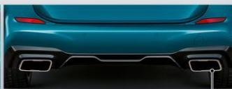
Exhaust system with  $\varnothing$  90 mm, twin tailpipes (four-cylinder models); BMW M235i xDrive with free-form tailpipes.
