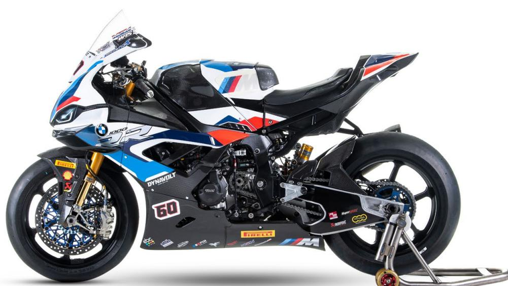
**Capacity/engine:** 999 cc, four-cylinder four-stroke engine with four titanium valves per cylinder and variable intake camshaft control BMW ShiftCam, liquid-cooled, titanium rods, 2-ring pistons
