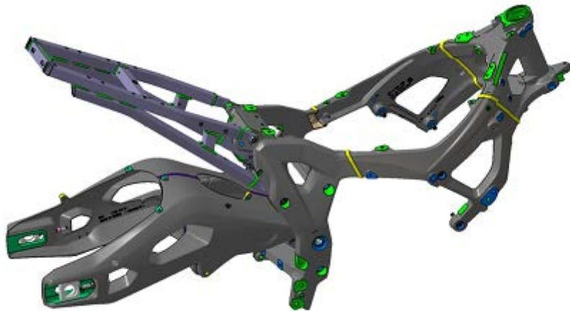
**New, much lighter Flex Frame with the engine more closely integrated in the frame as a load-bearing element.**
