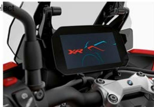
As is the case with the version for the supersports model, the variety of information, display quality and not least the user-friendliness of the new instrument cluster are currently unmatched. The new S 1000 XR, in conjunction with the BMW Motorrad Connectivity App, already comes as standard with practical arrow navigation and multiple waypoint guidance in the display.
