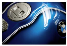
multiple masking and finish on the fuel tank.
