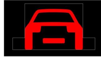
The **second warning level** (TOR2) is displayed if the system detects a dangerous situation in which the distance control cannot ensure the required minimum distance even at maximum permitted brake actuation (ACC must not activate emergency braking). Any abrupt possible braking manoeuvre of the vehicle in front is taken into account. ACC continues to carry out any necessary braking, but the rider has to be ready to brake and if necessary must brake to avoid a collision.
