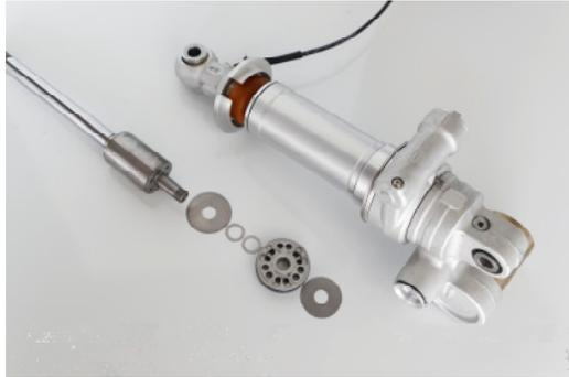
The DDC damping valves in the predecessor model were connected in series. The volume flow passed through the conventional and electrically adjustable damping section. Conventional damping was the lowest level of damping available. The electrical DDC valve increased damping. However, this resulted in the familiar drawback that the compromise between comfort and high damping tended to cause underdamping and pumping of the suspension.
