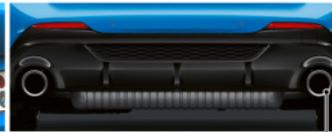
Twin-tailpipe exhaust with  $\varnothing$  90mm (four-cylinder models); BMW M135i xDrive  $\varnothing$  100mm, angle-cut.
